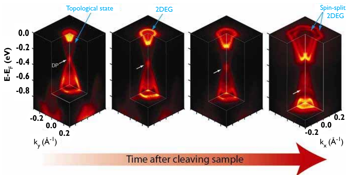
Figure 1: Electronic structure of \text{Bi}_2\text{Se}_3 , obtained using time-of-flight ARPES at increasing times after cleaving the sample ( h\nu = 19.2 eV).
